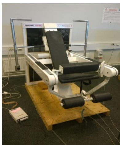
FIGURE 19. Modified David 200. Used for isometric knee extension and isometric knee flexion.
