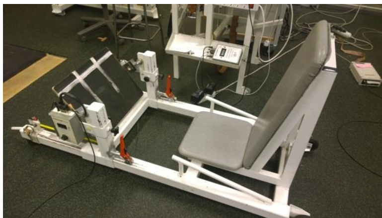
FIGURE 18. Isometric horizontal bilateral leg press, designed and manufactured by the Department of Biology of Physical Activity, University of Jyväskylä, Finland.
