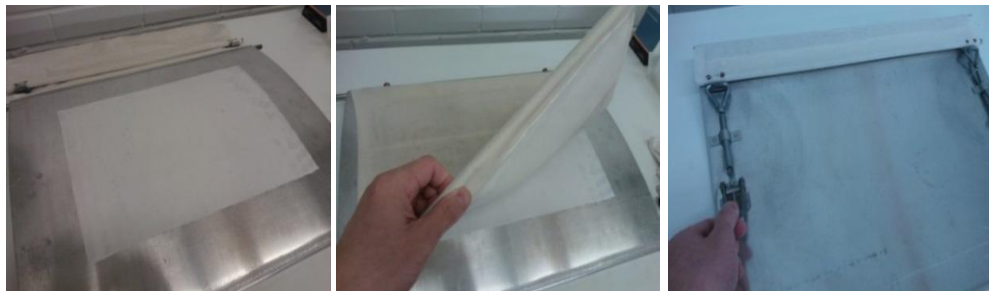
Figure 3.5. The drying process of a foam-formed handsheet.
