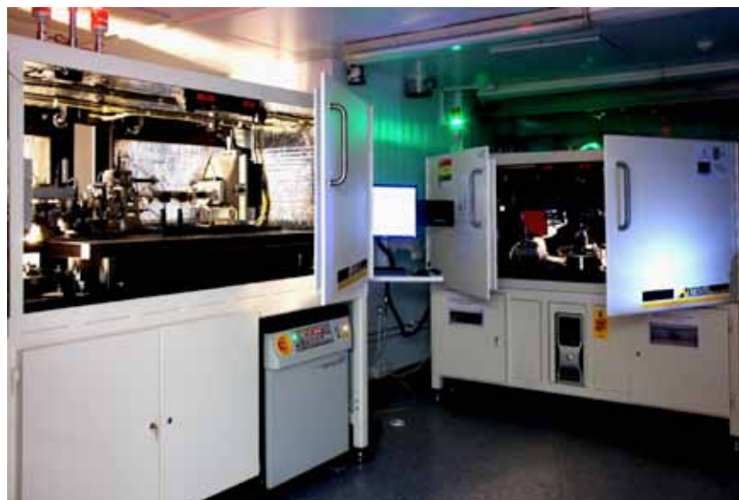
Figure 1. Xradia Multiscale X-ray tomographic facility. A microtomograph (right) and a nanotomograph capable of 50 nm resolution (left).
