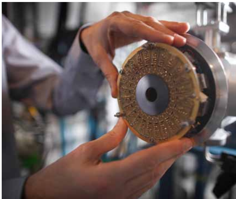
Fig. 3. The SPEDE detector mounted at the target position of RITU for the first in-beam test.
