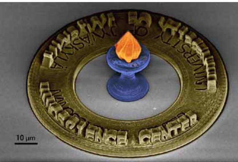
Fig.3. SEM image of a structure fabricated with the 3D lithography tool at NSC.
