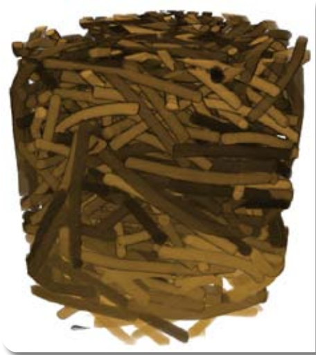
Fig. 6. A segmented image of a granular pile of short cut spaghetti. Tomographic imaging and fibre segmentation enables an accurate measurements of properties of the granular pile, e.g. the distribution of contact numbers.
