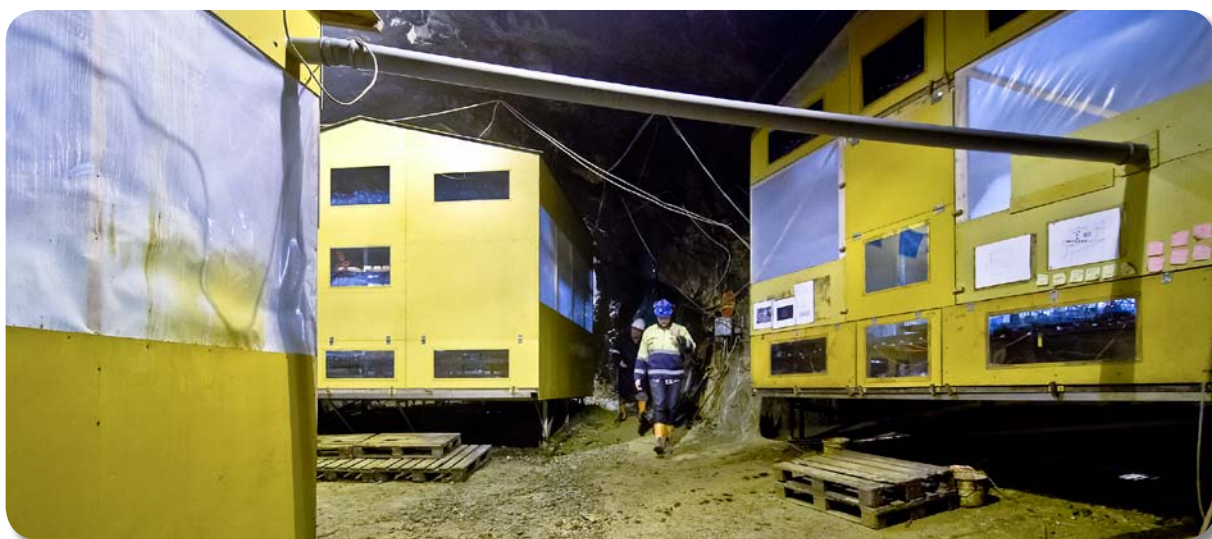
Three central tracking stations of the EMMA experiment (from left: F, G, and C). Each station is equipped with three double layers of drift chambers and connected to the data acquisition.
