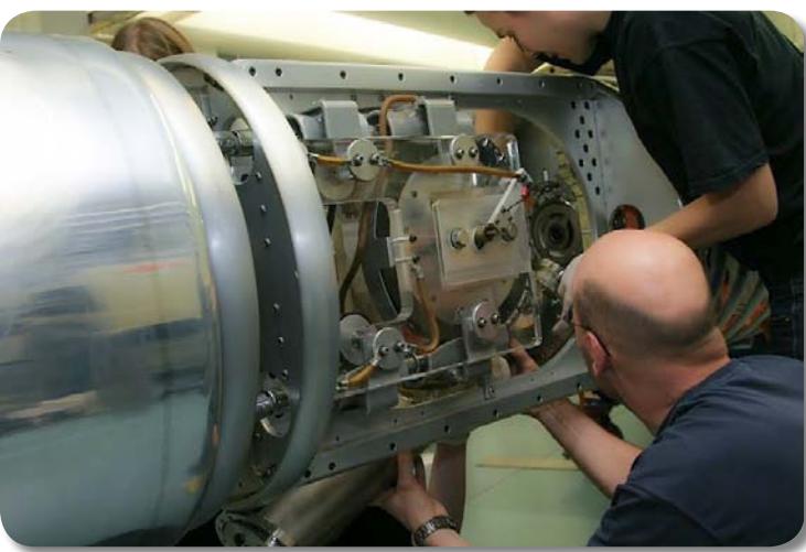
Fig. 1. The new stripper channel is being installed to the Pelletron terminal.
