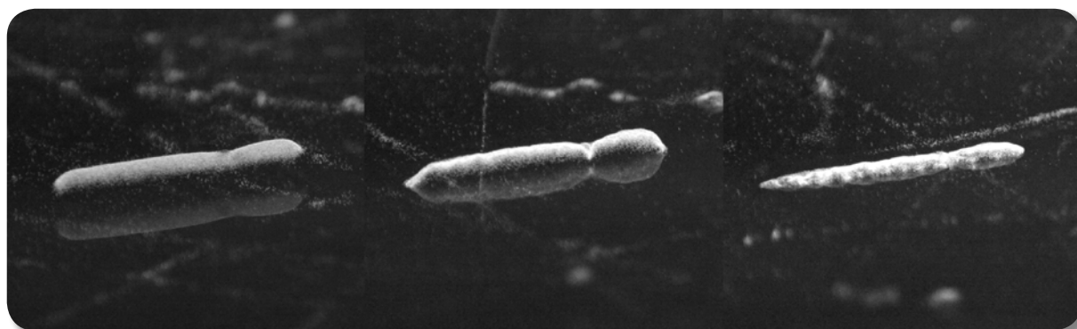
Fig. 4. Evolution of a single \alpha -particle and several \beta -particle tracks photographed in the JYFL cloud chamber.
