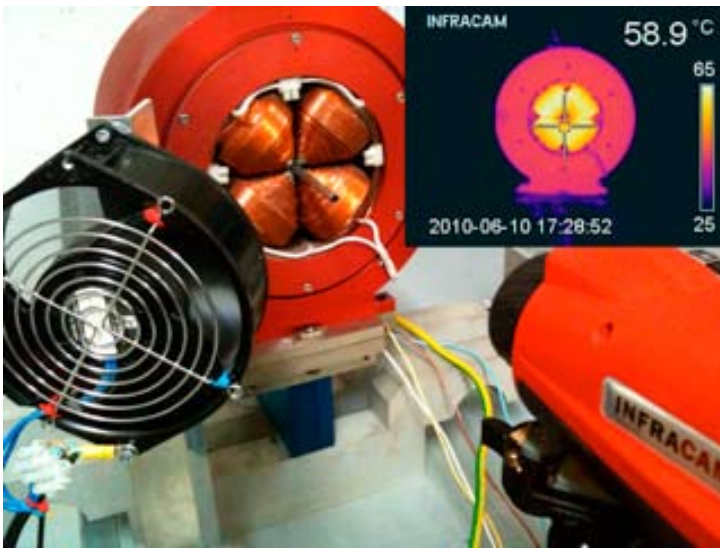
Fig. 1. Thermal testing of the quadrupole doublet microbeam lens.
