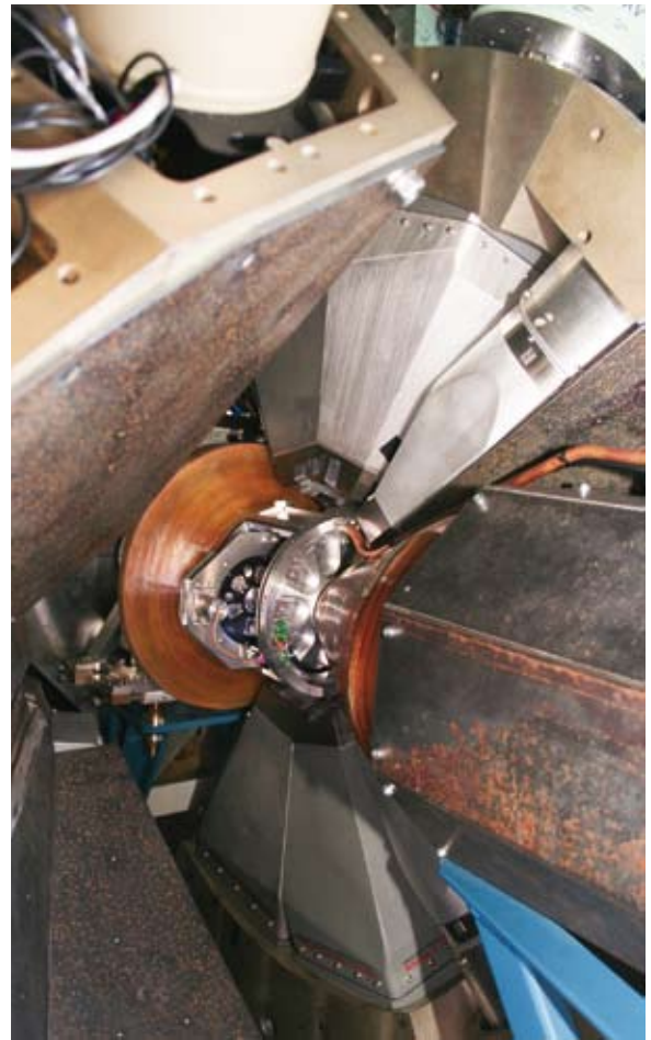
Fig. 2. The SAGE magnetic coils and target chamber combined with JUROGAM II detectors at RITU.
