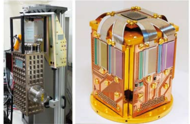
Fig. 2. Left: A novel cryogenic X-ray spectrometer based on an adiabatic demagnetization refrigerator (ADR). Right: A photograph of the 50 mK stage with the detector array chip and SQUID readout electronics.
