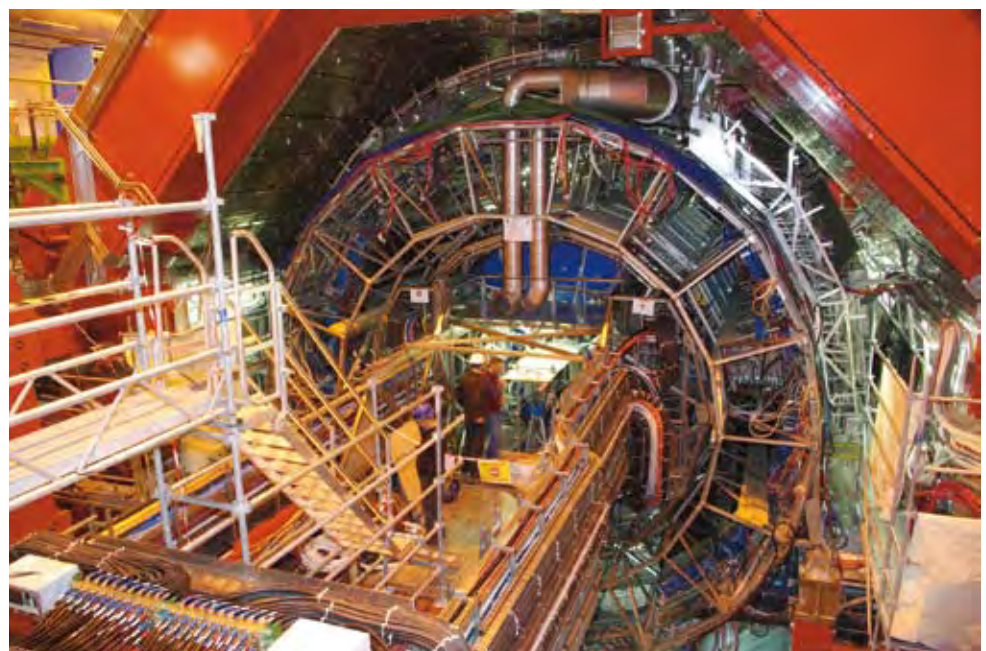
Fig. 1. Installation of T0 detector in the central region of ALICE
