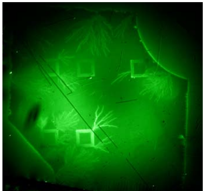
Fig. 4. Flux penetration into an epitaxial NbN film measured by magneto-optical imaging. Image courtesy of T. Johansen, Oslo University.
