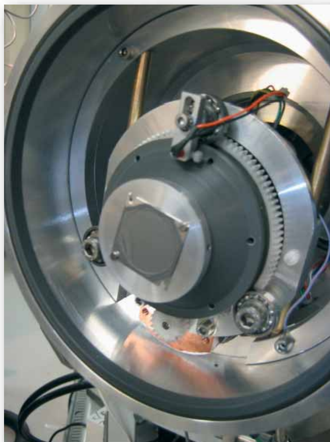
Fig. 2. The IReS Strasbourg rotating target wheel system installed at JYFL.
