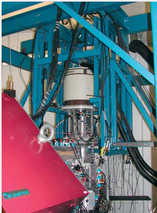
Fig. 1. A high efficiency segmented Germanium CLOVER Detector with Compton suppression installed into the new supporting frame at the focal plane of RITU separator.
