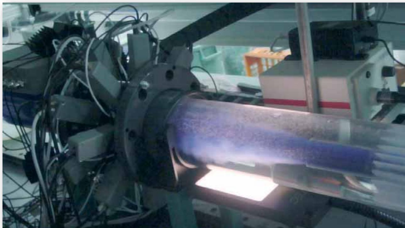
Fig. 1. Optical tomographic device mounted in concentric mixing tube of fibre suspension (dyed blue and discharged axially at the center of the tube) and water (annular flow) for measurement of consistency distribution in the mixing zone. In the actual experiment, unlike shown here, also the water phase is made opaque by added latex.
