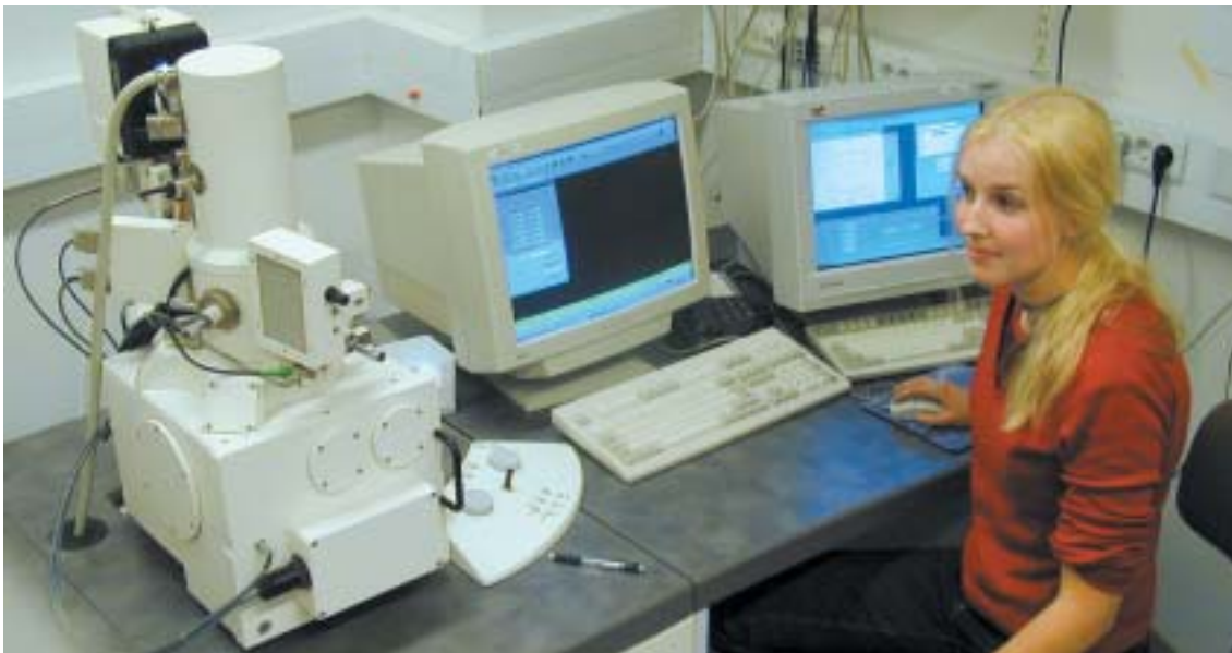
Fig 6. The fabrication of microelements with a scanning electron microscope in progress.
