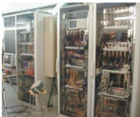
Fig 2. The TDR system housed in 3 air-conditioned racks in the RITU cave, instrumenting over 400 spectroscopy channels.
