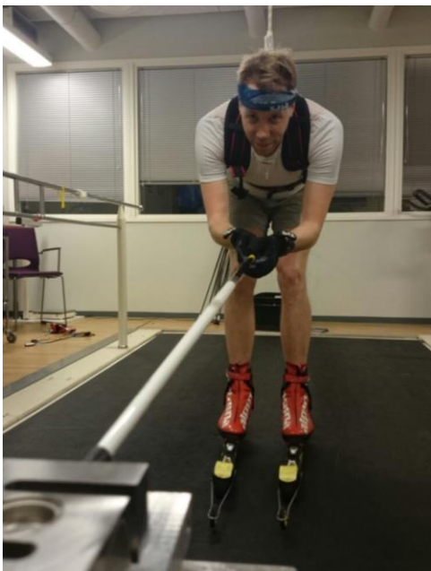
FIGURE 19. Determining the coefficient of friction value on the roller ski treadmill.
