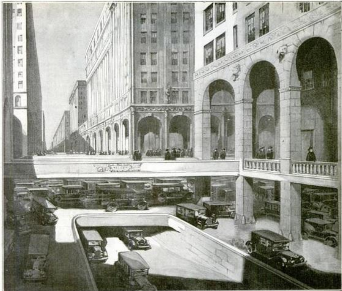
Triple-deck street corner in the crowded city of the future—a solution of the ever-increasing traffic problem proposed by Harvey Wiley Corbett, president of the Architectural League of America. Streets would cross one under the other, thus eliminating cross currents of vehicular traffic. Pedestrians would use an elevated sidewalk, bridged at all streets in both directions, ending the clash of foot and wheel traffic
