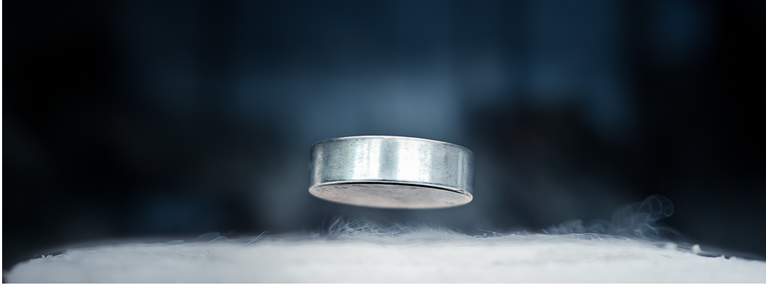
Figure 1.1: A permanent magnet levitating on top of a superconductor, the Meissner effect.
