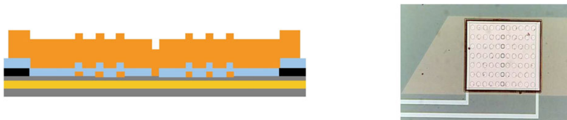
Fig. 2 (Color online) Left : schematic cross-sectional view of the device. Orange : Cu absorber and dots, blue : SiO x insulator, gray : Ti layers, yellow : Au layer, black : Nb contacts. Right : optical micrograph of the TES. The size of the Ti/Au TES is 186 \times 150 \mu\text{m}^2 and it is on a 1 \mu\text{m} thick SiN membrane fabricated on Si (110) surface
