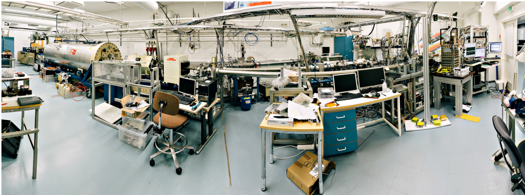
Figure 6.1: Photograph of the accelerator lab. On the left is the Pelletron accelerator. In center of the frame are the different beamlines and on the right is the TES setup connected to the target chamber.
