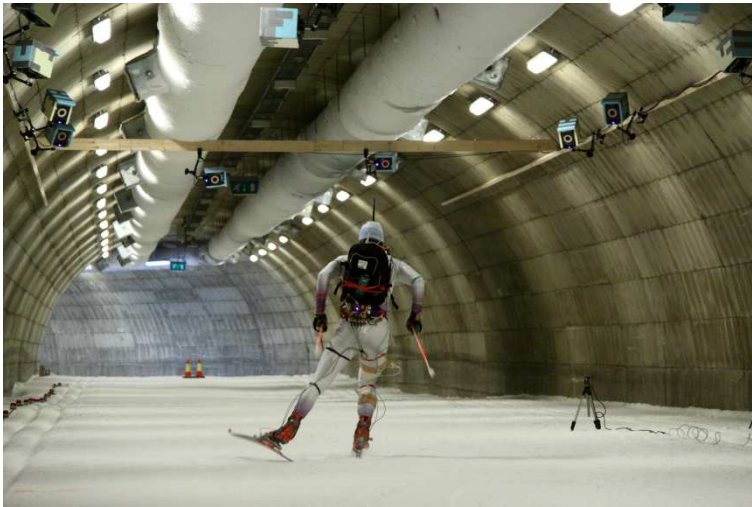
FIGURE 1. Measurement setup. Infrared cameras were attached to the rail in the tunnel. Measurement setup (13.2kg) was carried in rucksack.
