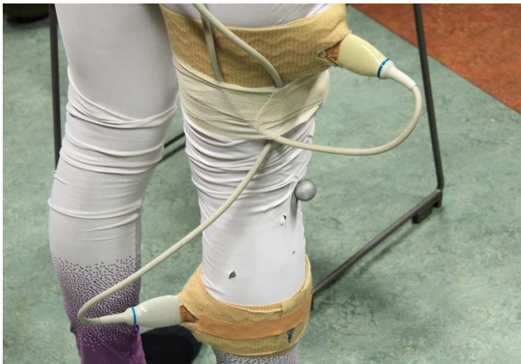
PICTURE 4. Attached probes for the MG and VL measurements. Ultrasound probes were firmly attached over the muscle belly.
