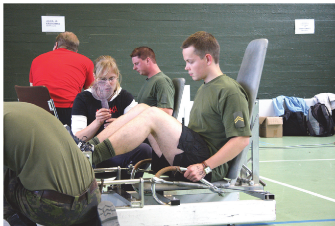
FIGURE 2 Bilateral maximal isometric leg extension measurement
