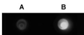
Figure 3. Gold (A) and silver nanoparticles (B) surface-modified with the same amount of Cyto633 fluorescent dye.
