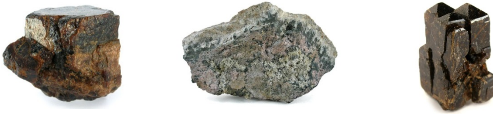
FIGURE 2 REE minerals from left: bastnasite, monazite and xenotime with rutile. 21-23
