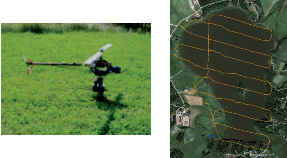
Figure 1. a) The FPI spectral camera in a helicopter UAV. b) UAV flight route over western basin of Petäjärvi
