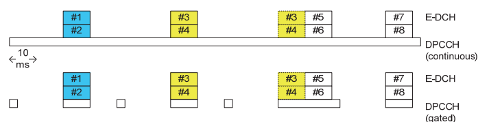
FIGURE 7 Illustration of VoIP transmission on E-DCH assuming 10 ms TTI and bundling of two VoIP packets into one TTI with continuous and gated DPCCH transmission.
