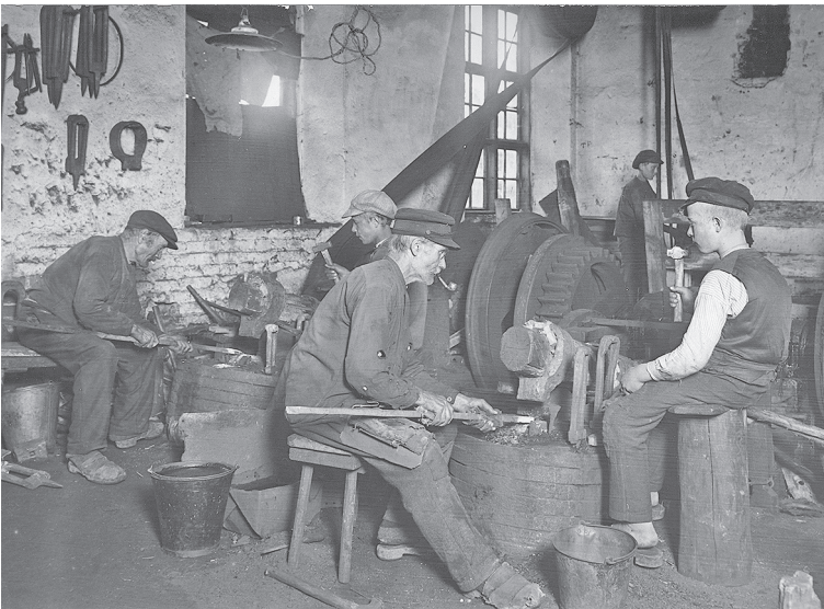
Figure 1. Young men from the Forstén and Forsberg smith families learning the nail-making trade in Strömfors Ironworks as informal apprentices in the 1920s. The working methods and organization of work had remained the same for hundreds of years. A. Ahlström Oy archives, Noormarkku. Used with permission.
