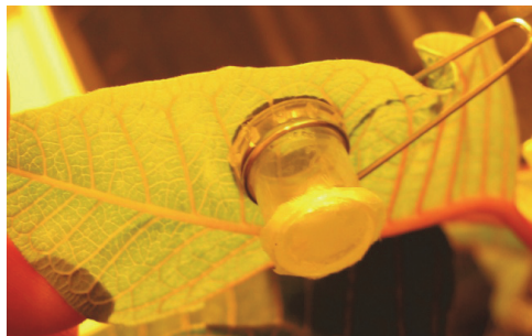
FIGURE 7 The clip cage designed for whitefly mating and production of larval cohorts used for spiromesifen bioassays.
