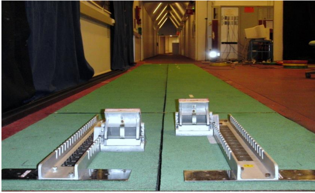
FIGURE 8. Position of the starting blocks on the force plates.
