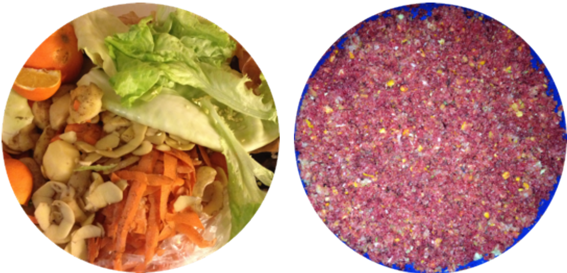
Figure 3. Manually sorted kitchen waste before (left) and after shredding (right) (Photo: Gossa Wordofa).
