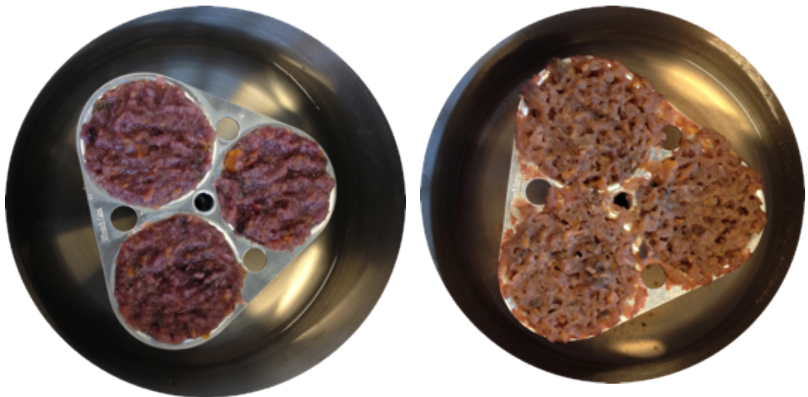
Figure 4. PC1 before (left) and after (right) pretreatment (PC1: Pressure-cooking with steam) (Photo: Gossa Wordofa).
