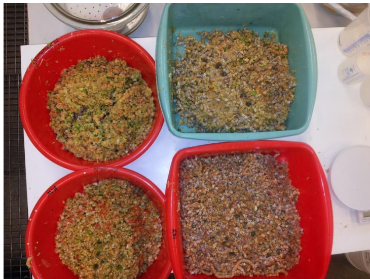
Picture 2 Grinded waste feedstock materials (Talsa W22). Food waste (right) and kitchen waste (left) (Photo: Jari Koponen).
