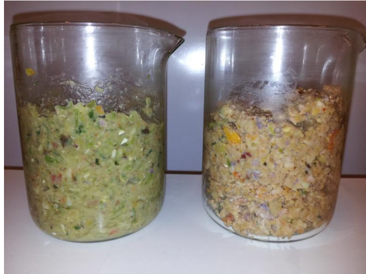
Picture 3 Food waste feedstock (right) and kitchen waste feedstock (left) after mixing the daily fractions. (Photo: Jari Koponen)
