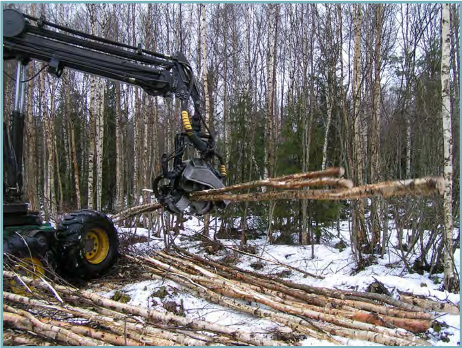
FIGURE 5. MTH multi-stem delimbed downy birch provides excellent energy wood for quality chips.
