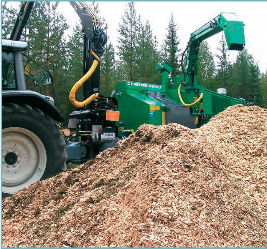
FIGURE 6. Large, tractor-driven chippers operated by an experienced entrepreneur often produce better chip quality.
