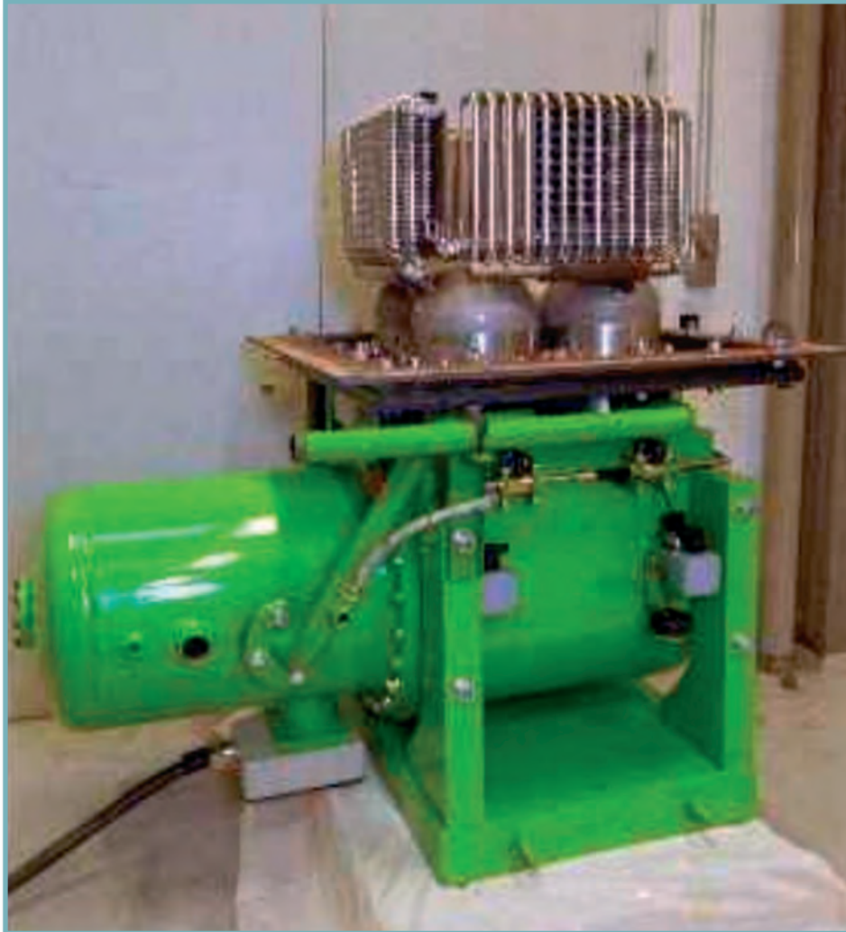
FIGURE 15. Stirling engine 35 kWe, before assembly. The heat transfer device is visible on the cylinder head. Photo: Stirling.dk
