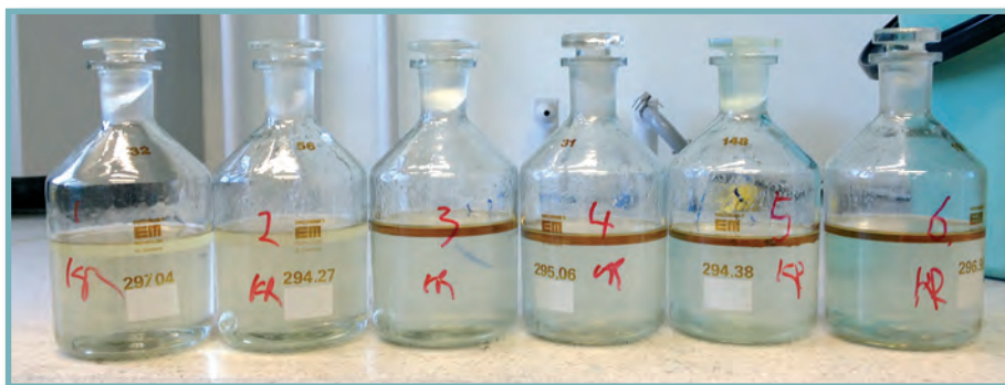
FIGURE 3. Extracted condensing waters from wood chips from biogasification with kerosene (1 and 2), pentanol (3 and 4) and hexanol (5 and 6).
