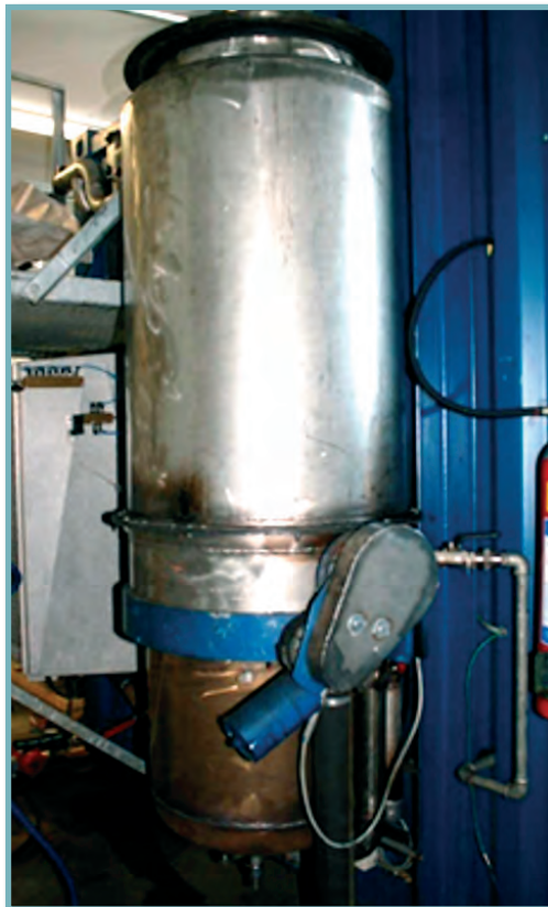
FIGURE 2. SOLO Stirling 161 micro CHP-module (9 kWe and 26 kWth) installed at the Centria renewable energy research laboratory (above) and Centria downdraft gasifier (left).
