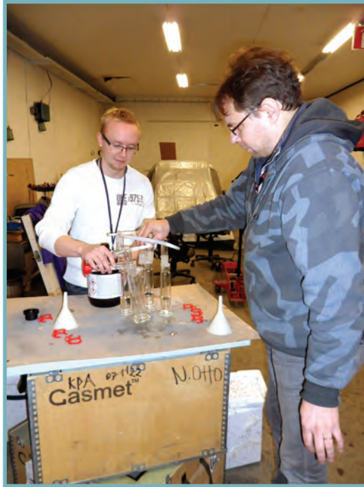
During the HighBio2 project researchers gathered several times to make measurements at different gasification plants. In the figure Jaakko Pulkkinen and Pekka Tynjälä prepared solutions used for tar analysis at a pilot gasification plant in Sievi in November 2012.
