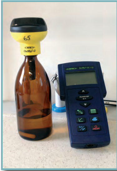
FIGURE 1. OxiTop Control system for biodegradation measurements in solution.
