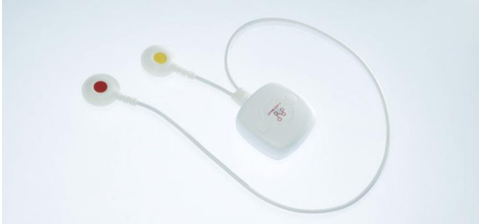
FIGURE 7. Firstbeat BODYGUARD RR interval recorder. (BODYGUARD 2013).
