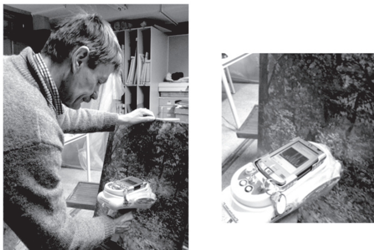
FIGURE 13 Head of material research laboratory Seppo Hornytzkyj demonstrates the prospects of using portable XRF-spectrometer in art attribution. Photos: Anna Hjorth-Röntynen
