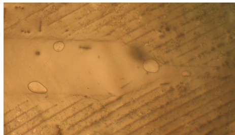
Figure 5.9: Simple microfluidic channel made by electron beam lithography combined with wet etching. The channel is enclosed with a coverslip. Its dimensions are 600\ \mu m and 100\ \mu m on the thicker and thinner section respectively. The channel is filled with water and some air bubbles are visible.
