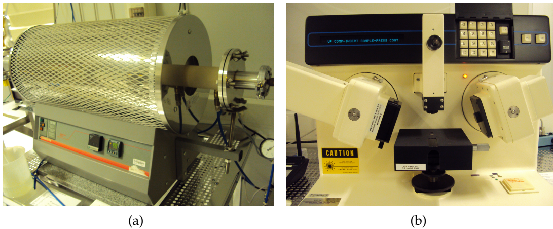
FIGURE 4.2 (a) Oxidation furnace used to oxidise silicon wafers. This instrument is equipped with a PID temperature controller. During oxidation the sample is placed in the mid of the chamber which is the hottest part of furnace. (b) Elipsometry equipment used to measure thickness of thermally grown silicon oxide.
