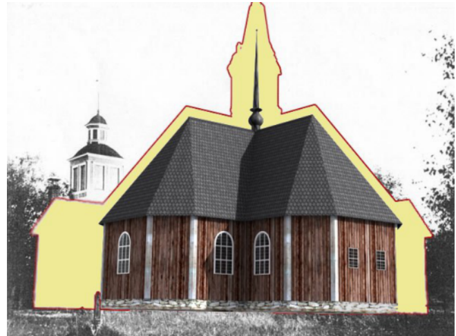
Figure 10. Overlay of the first phase. The yellow area presents the current size of the church.
