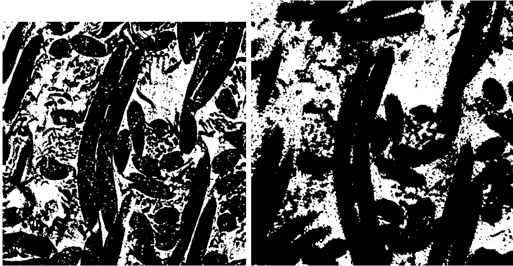
Figure 14: Tomographic images of dry (on the left) and wet press felt after segmentation.
