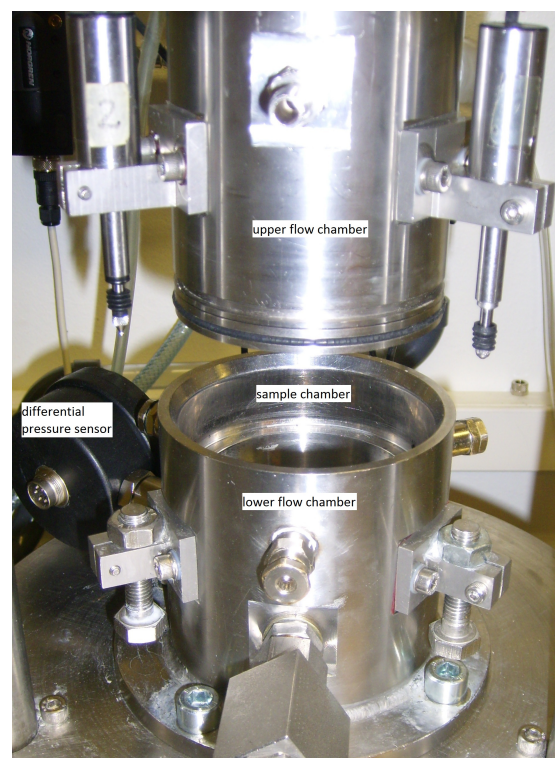
Figure 9: A close-up of flow chambers and differential pressure sensor.
