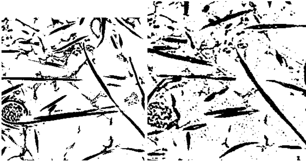
Figure 16: Tomographic images of dry (on the left) and wet synthetic chammy after segmentation.
