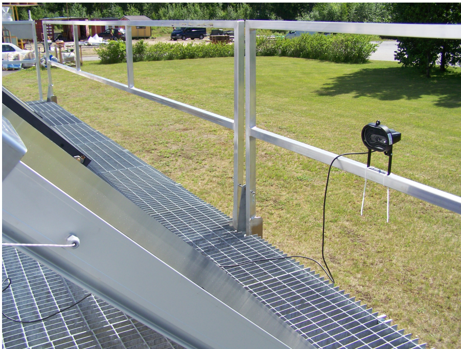
Figure 16: A photograph of the webcam in its final position on the railing in front of the collector; the cam is directed at the lower part of the collector
