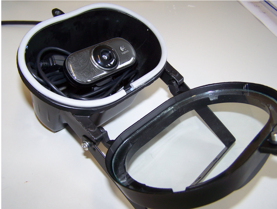
Figure 15: A photograph of the webcam inside the open halogen lamp casing
