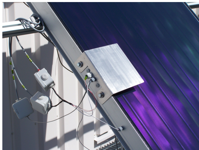
Figure 14: A photograph of the shading plate mounted on the collector's side
