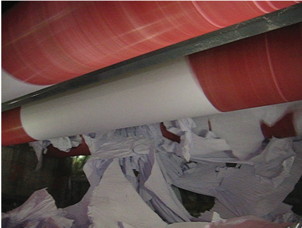
FIGURE 1 The stability has been lost and the web starts to break. (Courtesy of Metso).
