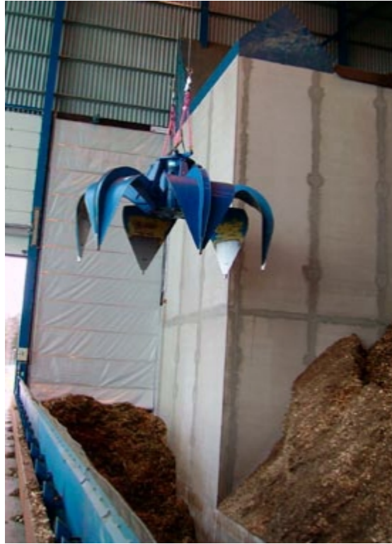
Figure 2.4: Grab crane system used in Mesto-Wärtsilä BioPower plants [13].
