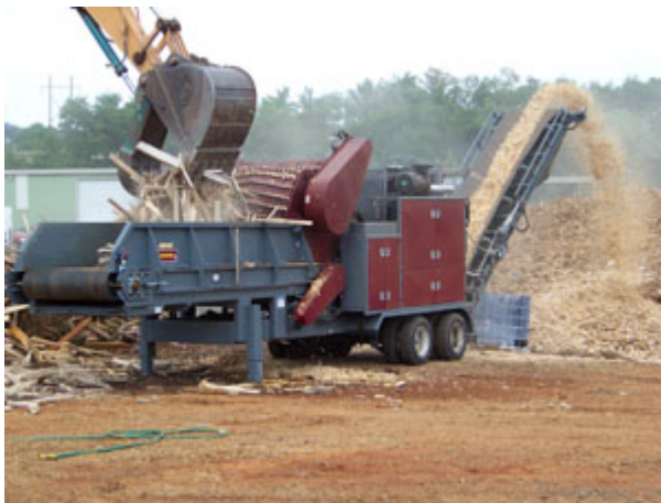
Figure 2.1: Dynamic 5240 horizontal grinder and hammermill [6].
