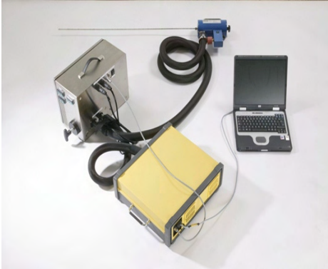
FIGUR 7. Centrias FoU FTIR gasanalysator Gasmeter Dx4000N.
