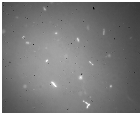
Figure 3.2 Typical image under fluorescence microscope of HiPCO SWCNT. The sample is excited with 659 nm and the nanotube structures with absorption close to resonance are visible with bright PL intensity.
