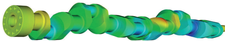
Fig. 7. The propagation of elastic waves in a crankshaft at f = 3 kHz. The color scale indicates the amplitude of the displacement, with blue corresponding to small displacement and red corresponding to large displacement.
