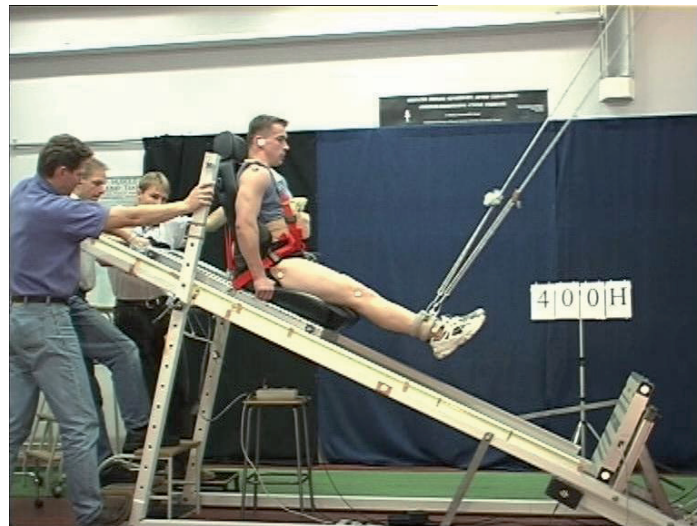
FIGURE 1 The sledge apparatus for jump test. The subjects' lower limbs were supported by a rope to minimize the metabolic fatigue of the quadriceps muscle group during the airborne phase due to the inclined leg position.
