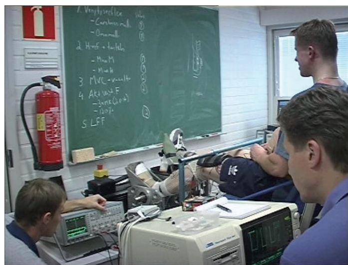
FIGURE 2 The ankle ergometer for assessing neuromuscular performance of the plantar flexor muscles.
