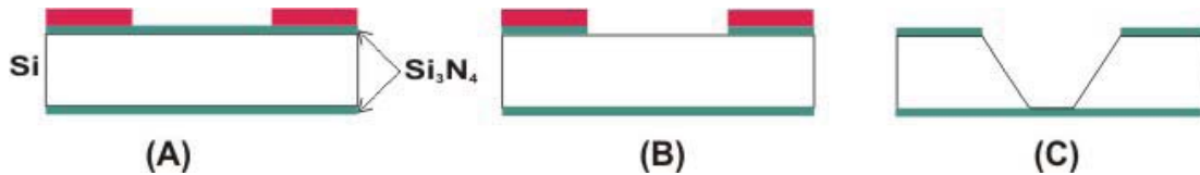
Figure 2.3 Fabrication of silicon nitride membranes by positive photolithography and wet etching of (100) silicon. (a) The chip after developing the photoresist (red) from exposed areas. (b) Silicon nitride (green) is removed with a reactive ion etcher. (c) Crystalline silicon is anisotropically wet etched in aqueous KOH. The etch rate is orders of magnitude slower in the direction of \langle 111 \rangle [6], resulting in the profile shown.
