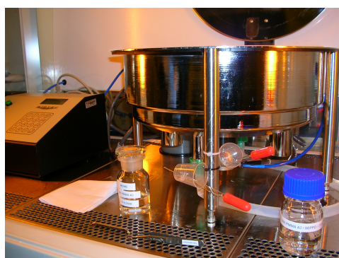
(b) Spinning the resists. The spinner is the same device that is used for the CNT deposition.
