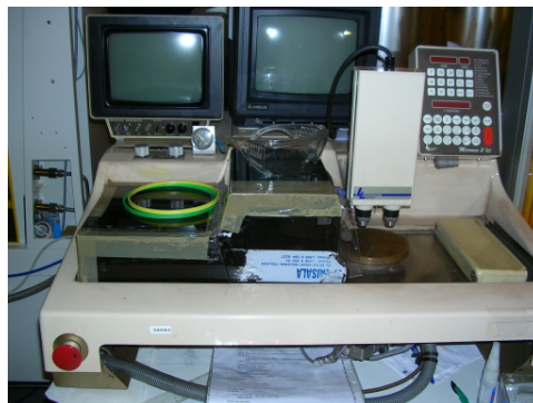
Figure B.1. The silicon saw which cuts the silicon wafer into chips.
