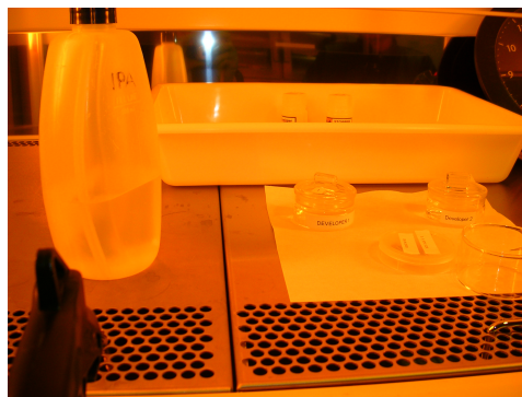
Figure B.5. The development instruments. Two solutions are needed: the first developer takes off PMMA 950 and the second removes PMMA 495.
