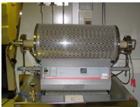
Figure B.2. The oxidation oven for oxidizing silicon and other naturally oxidized materials.
