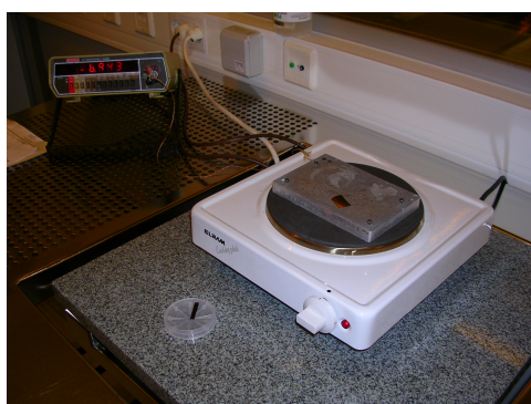
(a) The sample is baked before, between and after spinning the resists.
