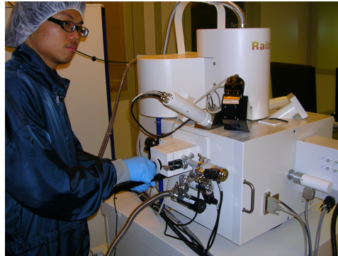
Figure B.4. Peerapong Yotranprayoonsak is using the Raith eLiNE for making the electrode pattern. eLiNE can also be used for imaging the samples.
