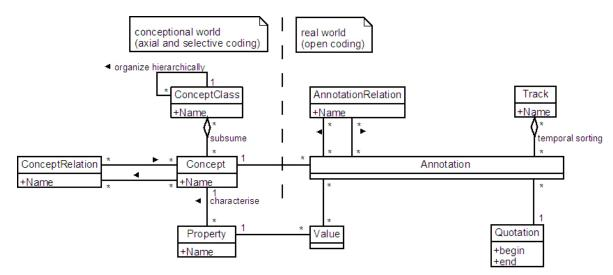
Figure 1. Complete metamodel of analysis results formulated as a UML class model. Boxes denote the various different kinds of elements occurring in our GT analysis results and the lines describe the relationships between them.
