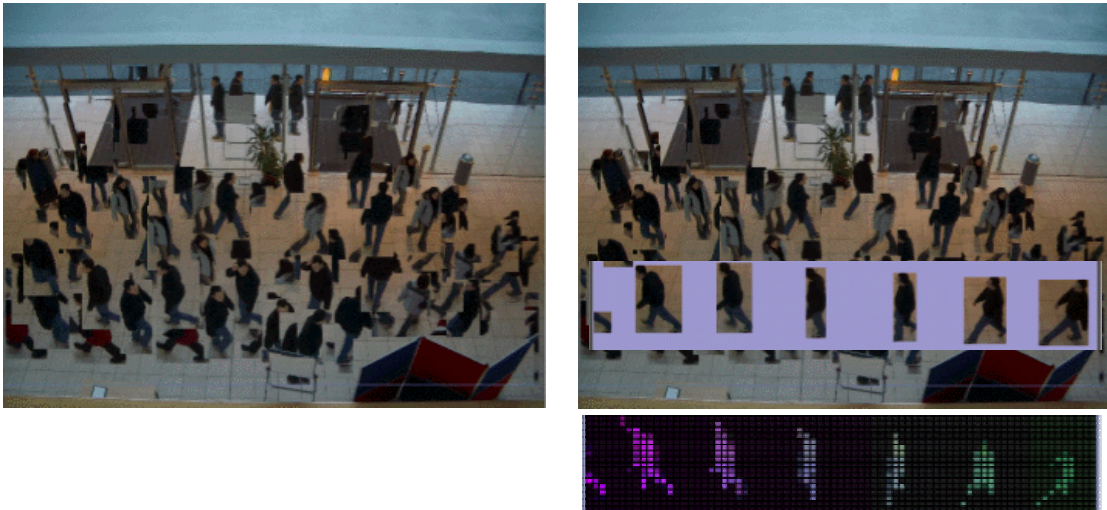
Figure 9. (top left) The video camera view of a foyer, composited with snapshots of activity; (top right) A tracking algorithm identifying the same person crossing the scene; (bottom right) Temporal ghost output created from the tracked figure.
