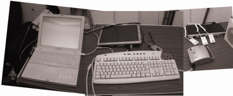
Figures 11a and b. The architecture illustrated in figures 11a and 11b was mainly designed and installed by Jennifer Sheridan and Nick Bryan-Kinn. As shown in figure 11a, it consisted of Tmote Invent artifacts installed in three of the chimes. These were programmed using TinyOS to send tilt information wirelessly to a central laptop located in a room next to the installation. When the motion of a person (or a breeze) was detected in a Tmote, the laptop triggered the playback of an associated audio track; when there was no interaction or wind, the associated playback was paused. Audio was wirelessly transmitted to these sensor chimes via three separate audio channels from the laptop PC. We used Max/MSP to control the sound without any noticeable lag in interaction. Figure 11b illustrates the actual laptop PC (left of image) and multichannel audio setup (right of image) used to drive the soundscape from the adjacent room (Mounajjed et al., 2007).
