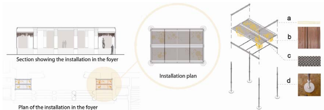
Figure 10. The image illustrates the process of designing and constructing Threshold . It shows early plan and section of Threshold situated in the foyer. The figure also illustrates the structure of the artwork including: a) planed wood, b) copper chimes, c) a metal mesh and d) a metallic structure.
