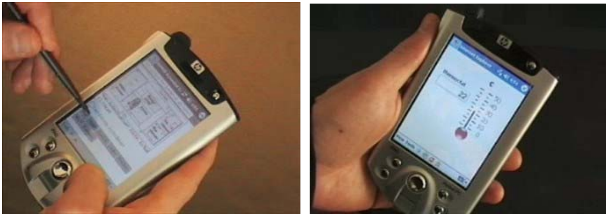
Figure 4. The PDA on the left shows a map of our mock-up apartment at our research center. The PDA on the right shows the current temperature in the living room of the apartment.
