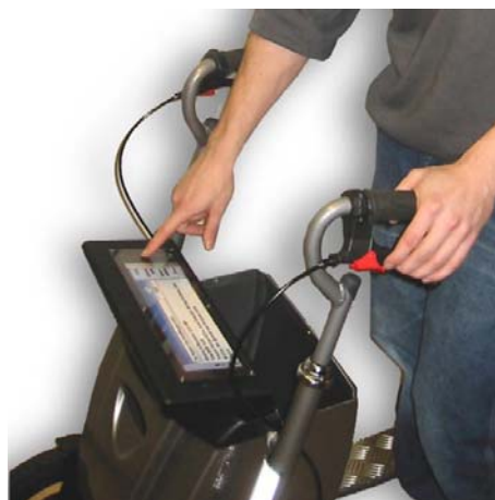
Figure 9. Mobility aids for older people were equipped with a multimedia terminal, making positioning-based outdoor navigation support possible. The project developed products and services to support the independent coping of older citizens. The ÄLLI project (Table 2, Technology J) concentrated on walking aids, user interfaces, and service concepts.
