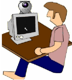
Figure 7. The Facial Mouse's working environment. The Webcam captures the user's movements that a software program translates in order to position the cursor on the screen.
