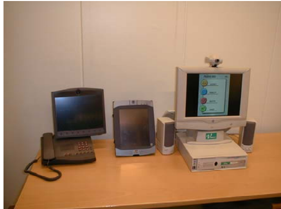
Figure 11. Various monitors, including TVs, and other components of the VT system were studied throughout the duration of the VT cases. Most recently (Case Two), the HomeHelper terminal device concepts, most of them at the “pre-products” stage, were tested. From the left: a special videophone set, a tablet PC, and a desktop PC.
