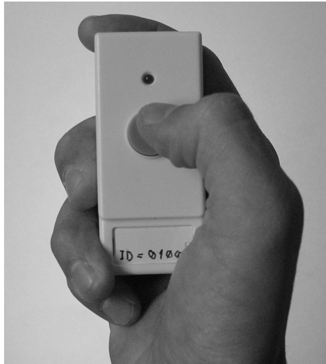
Figure 1. EventTagger is a wireless button that upon pressing sends a signal to the host PDA to gather and record all available context information into a log entry.
