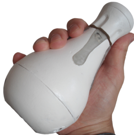
Figure 1. The Wigo: a tangible interactive device responding to manual activity patterns with haptic feedback. (Image used with permission from Bruns, Keyson, & Hummels, 2008.)
