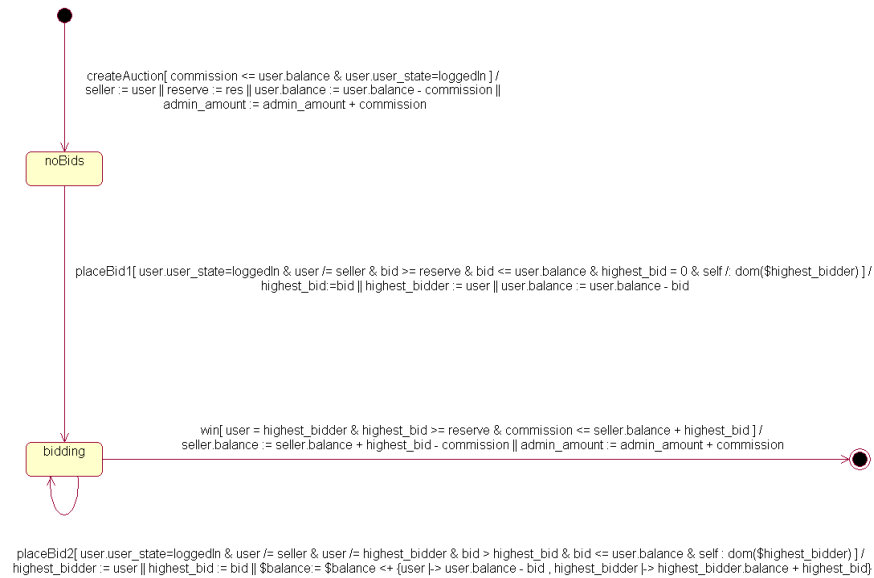
Figure 2. An example of a Statechart diagram of UML-B.
