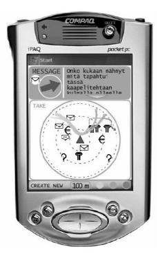
Figure 3. InfoRadar is a radar-like user interface to location-based messaging.
