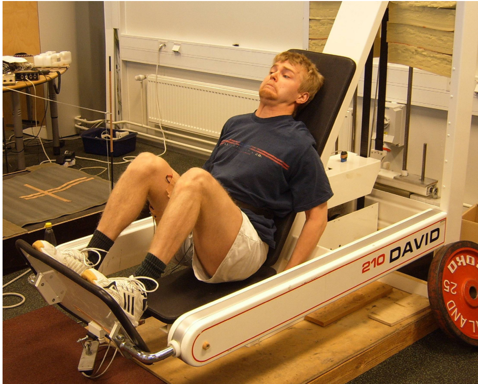
FIGURE 8 Experimental resistance exercise bout with David 210 system. Concentric leg-extension 1RM was tested with this device.
