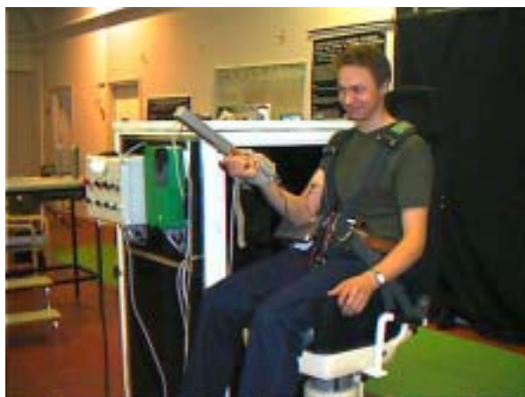
FIGURE 5 The ergometer subject system for recording eccentric, concentric and isometric forces for elbow flexors. The lever arm position can be changed for similar measurements for the knee joint.
