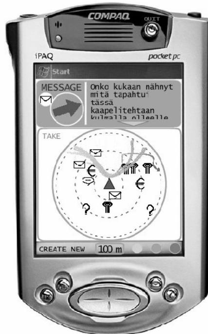
**Figure 3.** InfoRadar is a radar-like user interface to location-based messaging.
